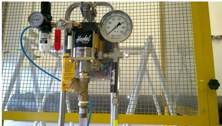
Hydrostatic test setup, with the casing placed inside a protective screen
