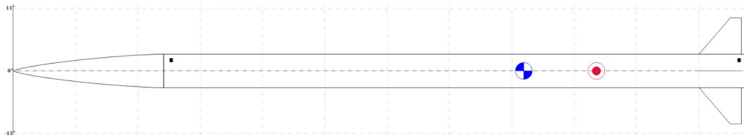
Figure 9 - Center of Mass (Blue) and Center of Pressure (Red) calculated with RASAero.
